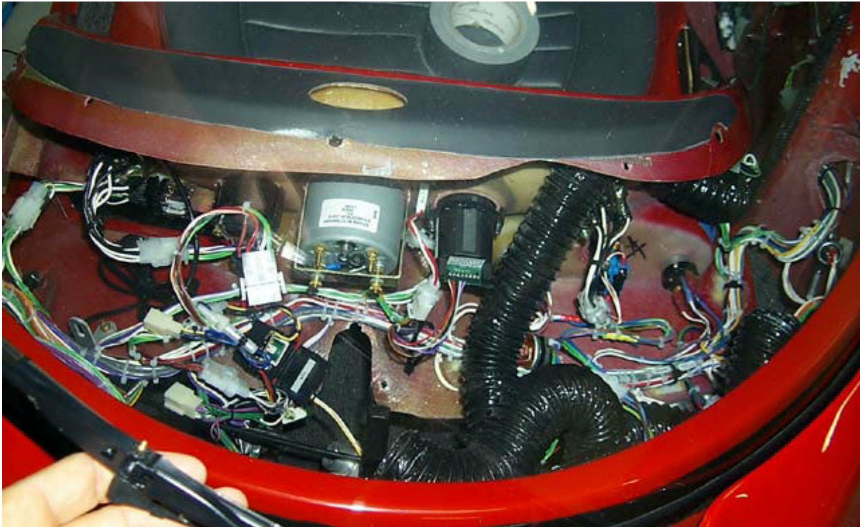
Dashboard removed, as seen through windshield.
